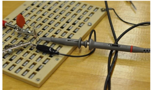
This is the probe set to 10x and a close up of the bulb and capacitor in parallel.
