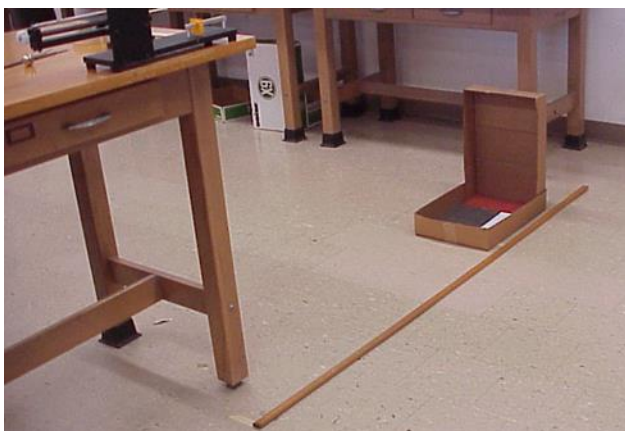
Figure 9 - Setup showing how to measure the horizontal reference distance D_r using masking tape on the floor. Fine cell graph paper is taped on the rubber mat in a cardboard box lid. Carbon paper placed face down on the graph paper leaves black impression marks where the steel ball lands.
