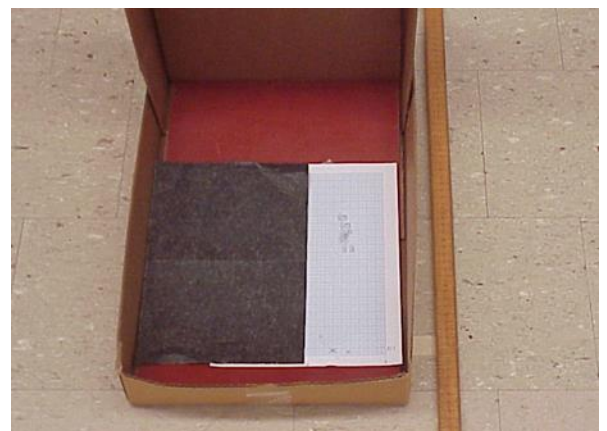
Figure 9 - Setup showing how to measure the horizontal reference distance D_r using masking tape on the floor. Fine cell graph paper is taped on the rubber mat in a cardboard box lid. Carbon paper placed face down on the graph paper leaves black impression marks where the steel ball lands.
