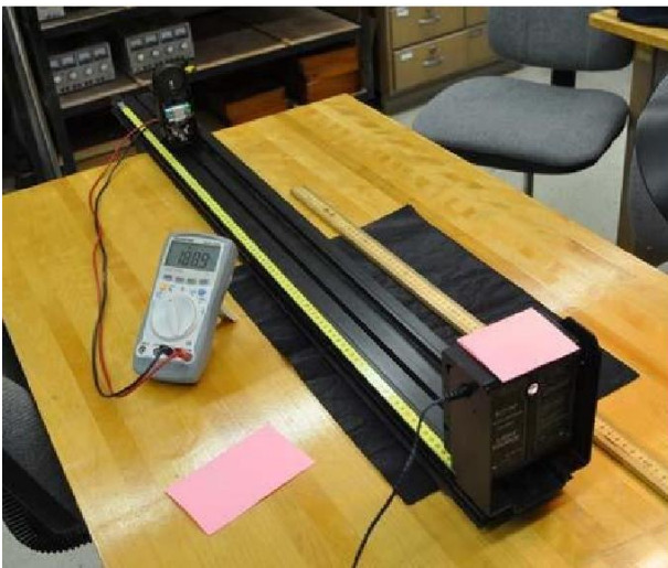
Left: Inverse square law apparatus showing Pasco light source and sliding optical sensor head on optical rail. Sensor head connected to DMM used in frequency counter mode (GW Instek GDM-396). Right: Close up of optical sensor head with TSL237 chip centered on circular light output from source.
