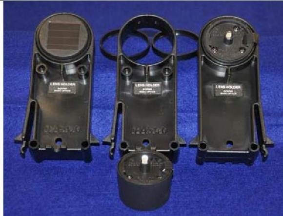
Solar path light white LED optical head mounted in PASCO Basic Optics lens holder. Left: Back side of optical head showing solar cell for charging battery. Center: Foreground shows optical head of the white LED solar path light. Background shows empty lens holder and two black plastic retaining rings used to mount the optical head. Right: Front side of optical head showing white LED with retaining rings installed.
